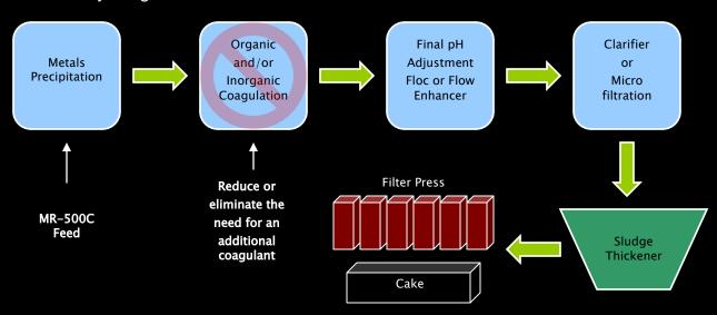
The DTC ion grabs the metal and releases the Ca. The Ca then pacifies any chelating or complexing materials. Any unchelated calcium, upon pH adjust, then coagulates through the co-precipitation of calcium hydroxide.
